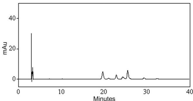
**Fig. 1.** High-performance liquid chromatogram of a methanolic extract of quinoa seeds (360 nm).
