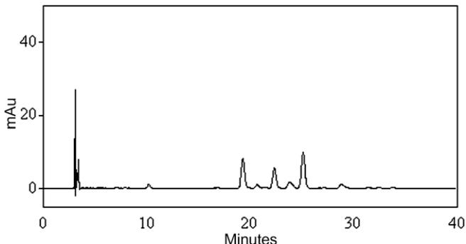
Fig. 2. High-performance liquid chromatogram of a methanolic extract of quinoa sprouted seeds (360 nm).
